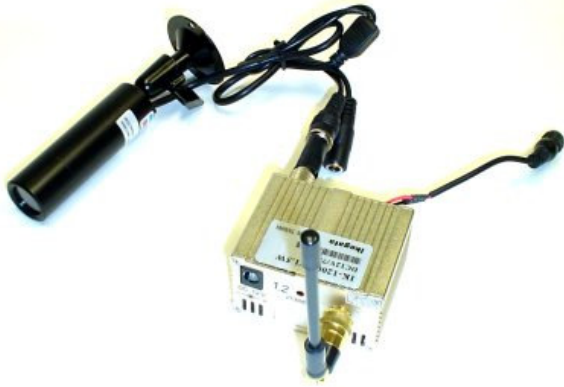
Room setup: PIR Motion sensor trigger, video camera connected to a wireless transmitter
