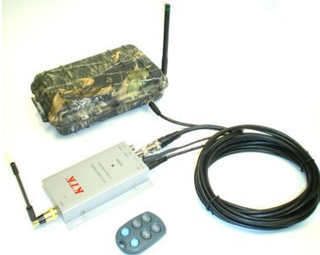
Recording Setup: Video receiver connected to the Trekker MiniDVR video input with manual KeyFob trigger
