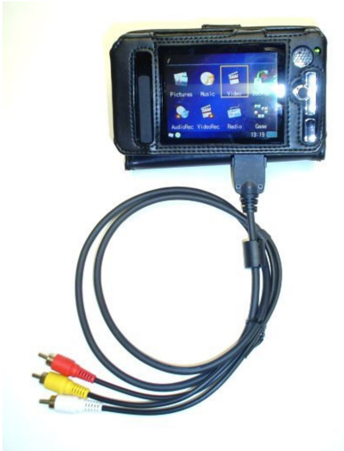
Connect the Video Input of the PVP to the Trekker MiniDVR Video Output for camera setup
