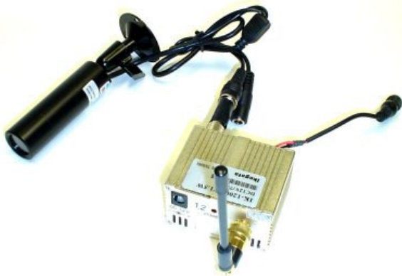
Room setup: PIR Motion sensor trigger, video camera connected to a wireless transmitter
