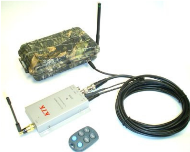
Recording Setup: Video receiver connected to the Trekker LANC video input with manual KeyFob trigger
