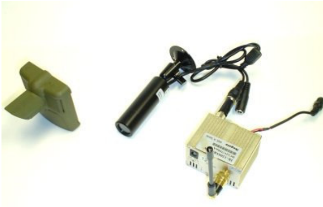
Room setup: PIR Motion sensor trigger, video camera connected to a wireless transmitter
