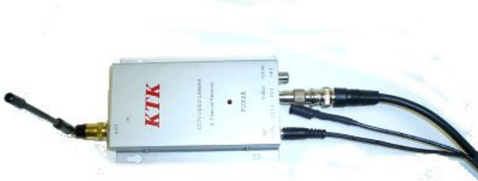
Recording Setup: Video receiver connected to the Trekker LANC video input
