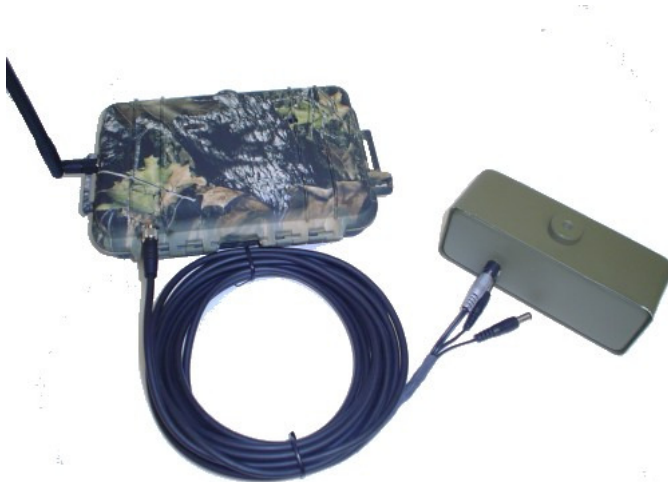
Figure 5: Connecting an IR Array to the Power Box for remote IR Illumination UndercoverEye HDD or Trekker units.
