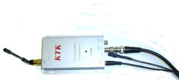
Figure 3: Connect the 2.1mm power connector from the video cable to the video receiver and the video input to the video output of the video receiver.
