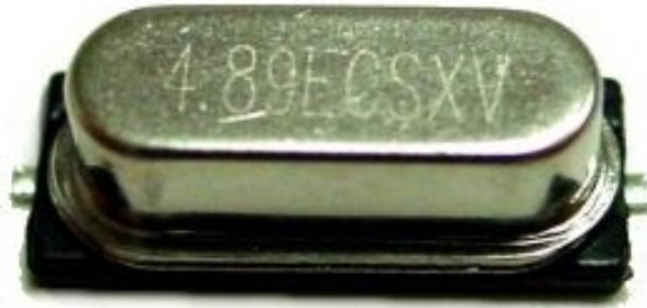
Figure 3: New 4.8970 MHz Crystal
