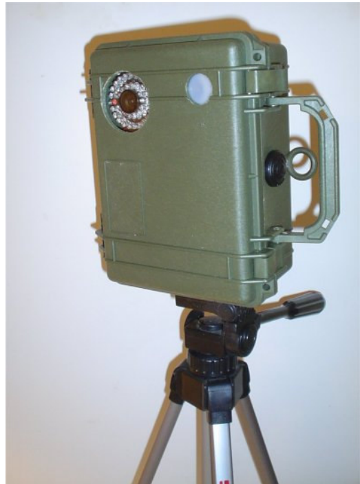
DVREye™ setup using a standard camera tripod
