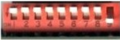
All switches "UP".
