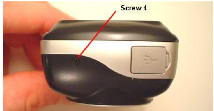
Remove screw 4 from the right side of the case.
