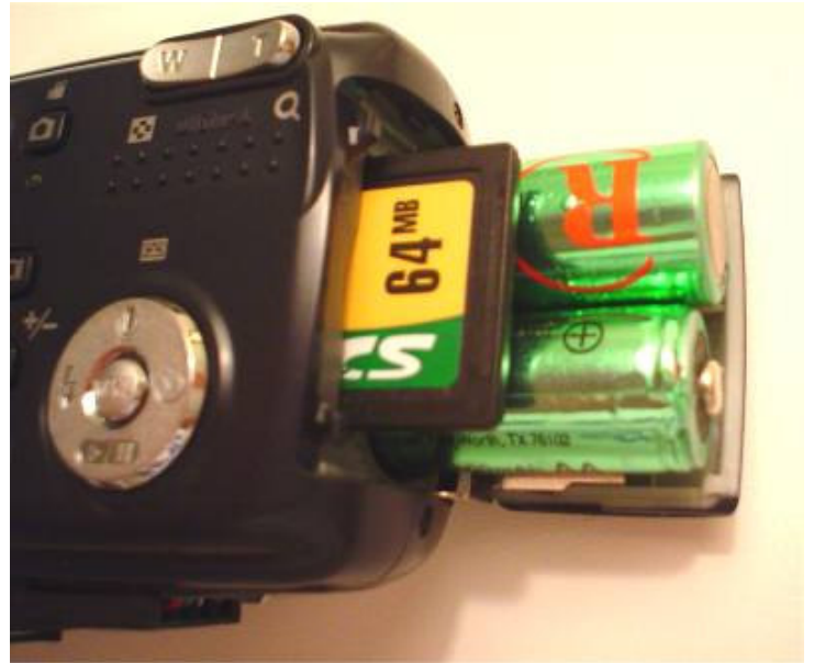
Remove the 2 AA batteries and Media Card
