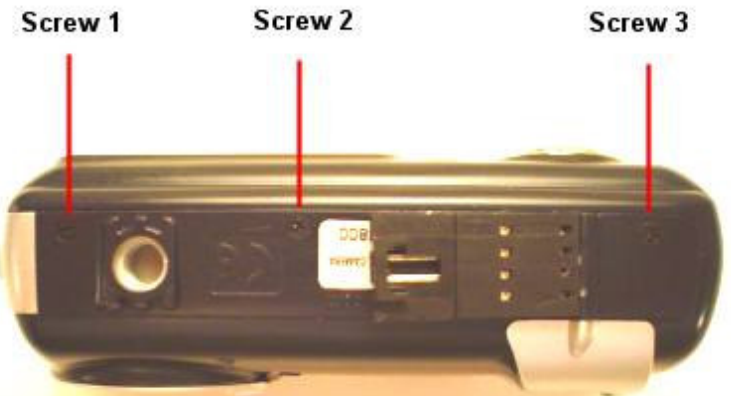
Remove screws 1,2, and 3 from the bottom of the camera case.
