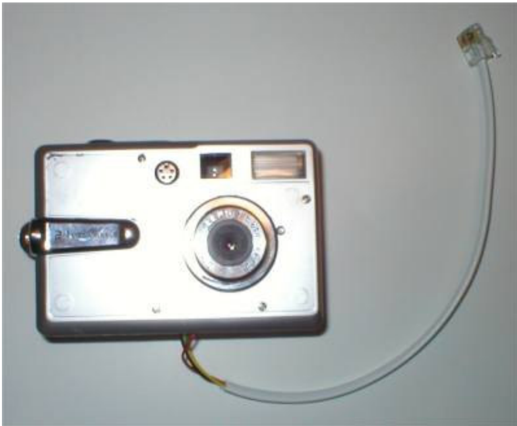
Completed Modification. This camera was wired using the phone cable for the PixController Universal board.
