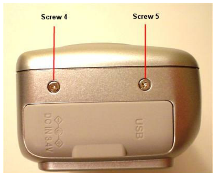
Remove screw 4 from the left side of the case.
